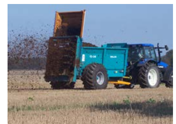
Pic 49. Vertical muck spreader spreading solid manure (Photo: Närke AB)
