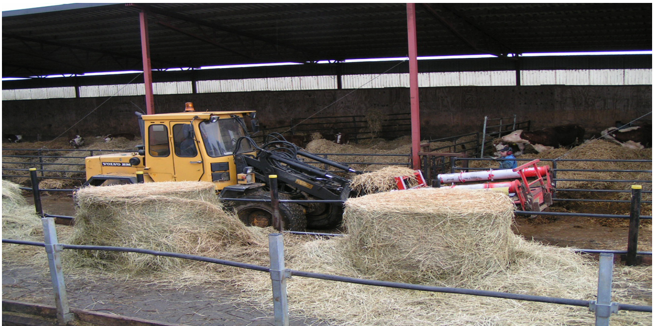
Pic 40. Using a tractor driven straw distributor makes the job of bedding for cattle easier.
