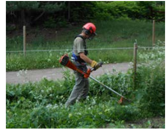
Pic 29. A brush cutter is a necessary tool to combat bushes and to mow down the grass under electric fences.
