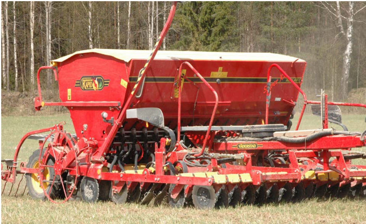
Pic 16. A specialized drill support seeding an existing grass ley without having to plough and harrow the land.
